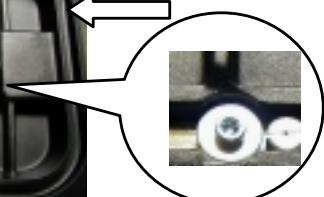
Fasten the vacuum handle with a washer and hexagon hollow head plug M8x30 and insert the foot sealing into the corresponding notch.
