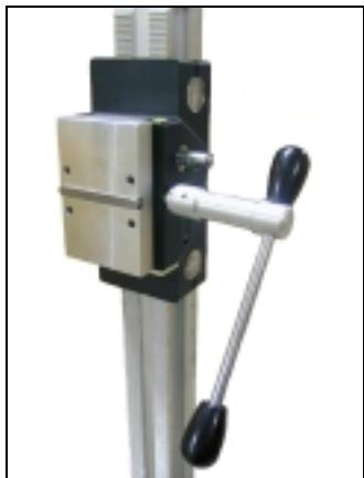
Move the tool mount with the attached core drill tool upwards until it locks in the final position.
