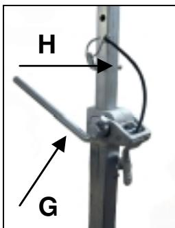
Position the drilling stand. Position the quick release fastener support as close as possible behind the support on the base of the stand. Fix the stand by turning crank (G) clockwise. Secure in position by means of the appropriate bolt (H).
