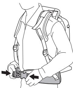
**CAUTION:** Make sure to release the hip belt buckle before unloading the blower.
