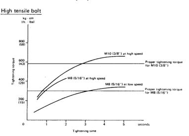
Hold the tool firmly and place the socket over the bolt or nut. Turn the tool on and tighten for the proper tightening time.
